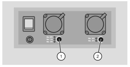
➤ Set the same flash energy using the arrow buttons (1, 2, 3, 4). The values to be set symmetrically can be found in the table (refer to Chapter "Setting the flash energy asymmetrically," Page 37).
