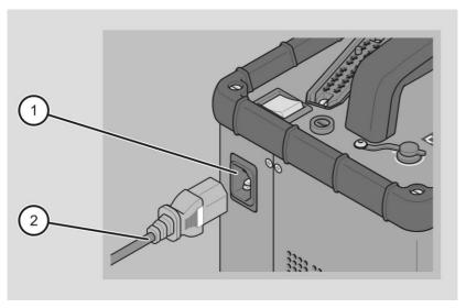
To remove the mains cable from the device, proceed as follows:
