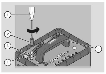
Two spare fuses are contained in the handle of the device. Remember to insert a new spare fuse as soon as possible.
